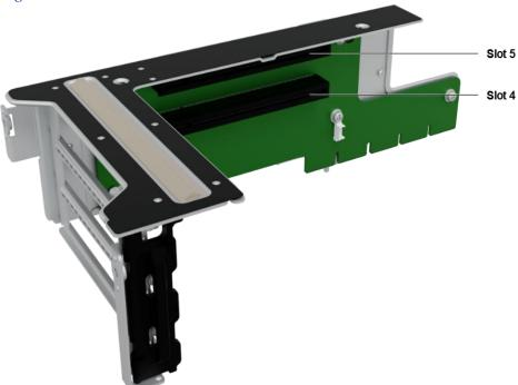
I/O module 3 → Figure 2-6 shows an SR3LB riser card installed in I/O module 3.
