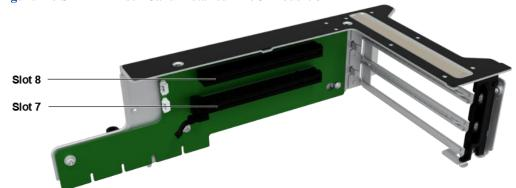
→ Figure 2-9 shows an RC0510L2A riser card installed in I/O module 3.
