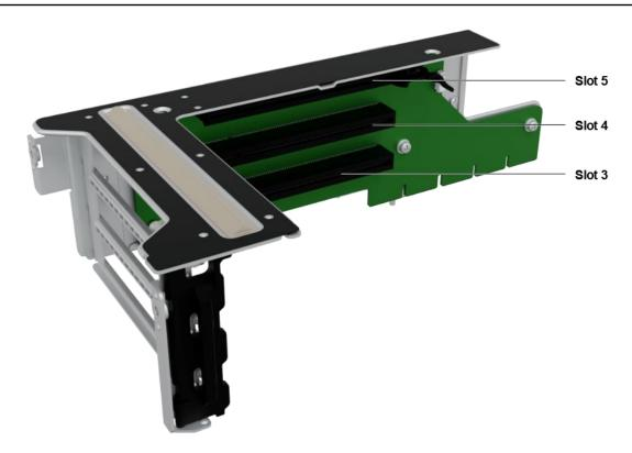
→ Figure 2-4 shows an SR2RB riser card installed in I/O module 2.
