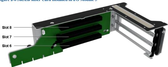
→ Figure 2-7 shows an SR2LB riser card installed in I/O module 3.
